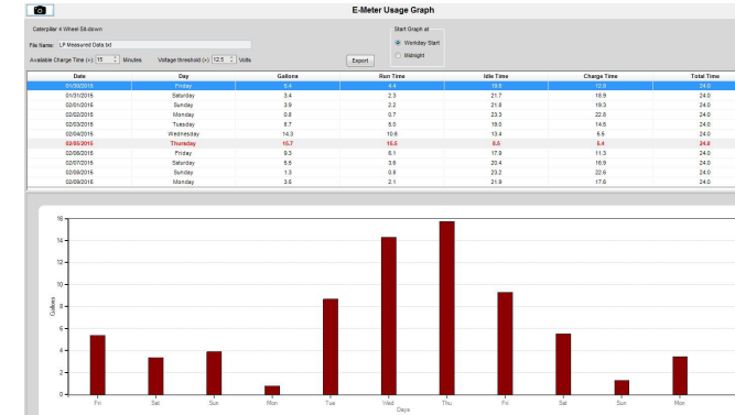
Figure 2. DAILY SUMMARY REPORT – The daily data report includes accumulated propane usage and run, idle and key off times.
