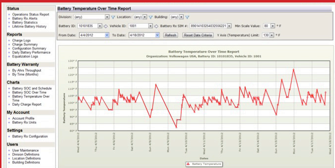
Figure 3. BATTERY TEMPERATURE CHART – Provides ability to review battery temperature in detail for any time period in the history of the battery.
